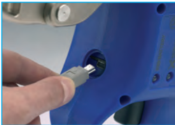
USB interface to trace the tool usage history.
