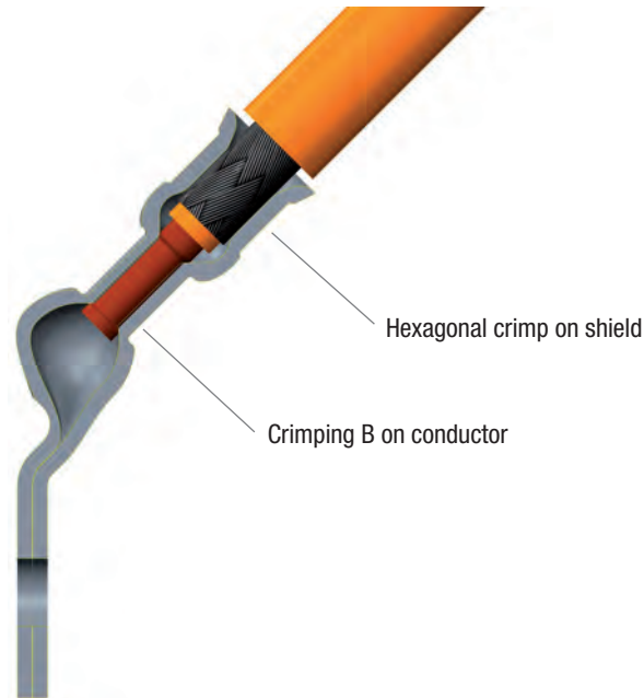
Conductor and shield termination
