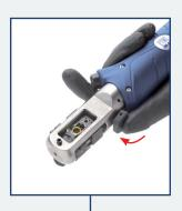
Release the die lever to automatically hold the lug between the dies.
