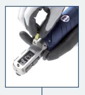
Insert the lug in the tool head up to stopper.
