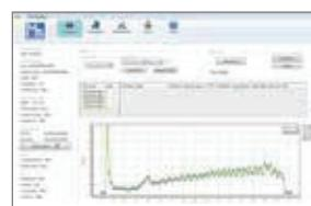
With this software, it is possible to configure the tool, record the crimping data and analyse the cycles already done.
