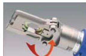
Nickel plated head rotates through 360°
