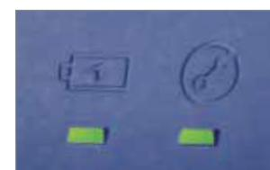
Service indicator lights informing about the battery charge level and service control if necessary.
