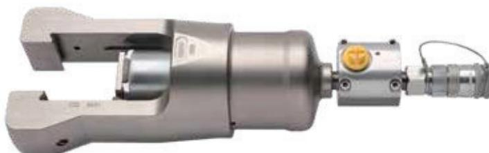
**3 colour LED indicator gives information about the hydraulic tool condition** (flashes 3 times after each crimping operation).
