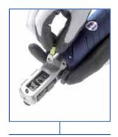
Insert the lug in the tool head up to stopper.
