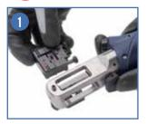
Secure pairing of die and stopper ensured by a disymetrical die guide.
