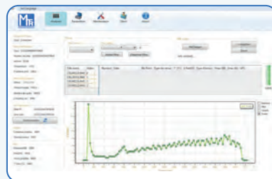
With this software, it is possible to configure the tool, record the crimping data and analyze the cycles already done.
